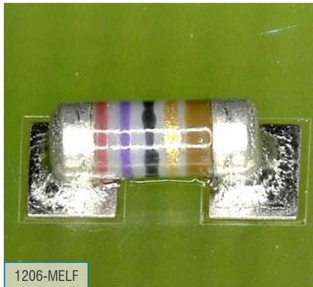
The flux residues of **FELDER ISO-Cream®"Clear"** SMD soldering paste have a very limited expansion (the flux does not flow over the edge of the solder resist mask). Thus the pseudo failure quote, especially with AIO-controlling systems, is significantly reduced, as reflecting flux residues could be interpreted as solder bridges (wrong).
