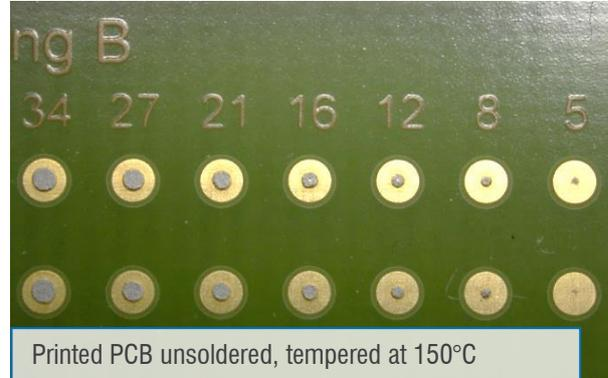
Printed PCB unsoldered, tempered at 150°C
