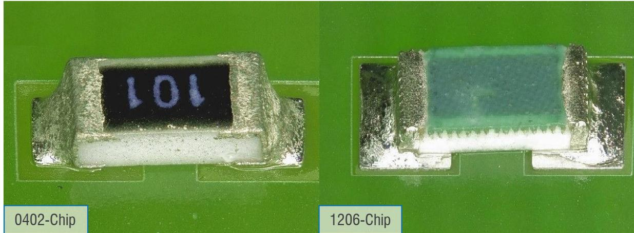
The solder paste ISO-Cream® "Clear" is insensitive against humidity and temperature. It shows no tendency for formation of solder balls at chip-resistances and capacitors. Excellent soldering results with clear flux residues with very high surface resistivity values.
